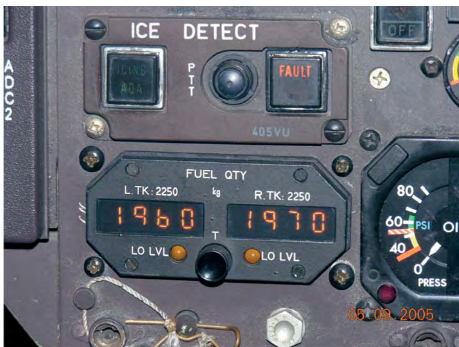
Photo 78: Indication given by an ATR 42 FQI fitted on an ATR 72 with a quantity of 3800 kg of fuel selected.
