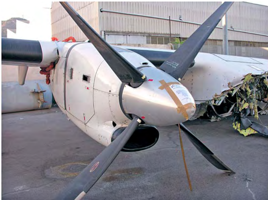
Photo 21: Right engine – note the propellers in the fully feathered position (red line).
