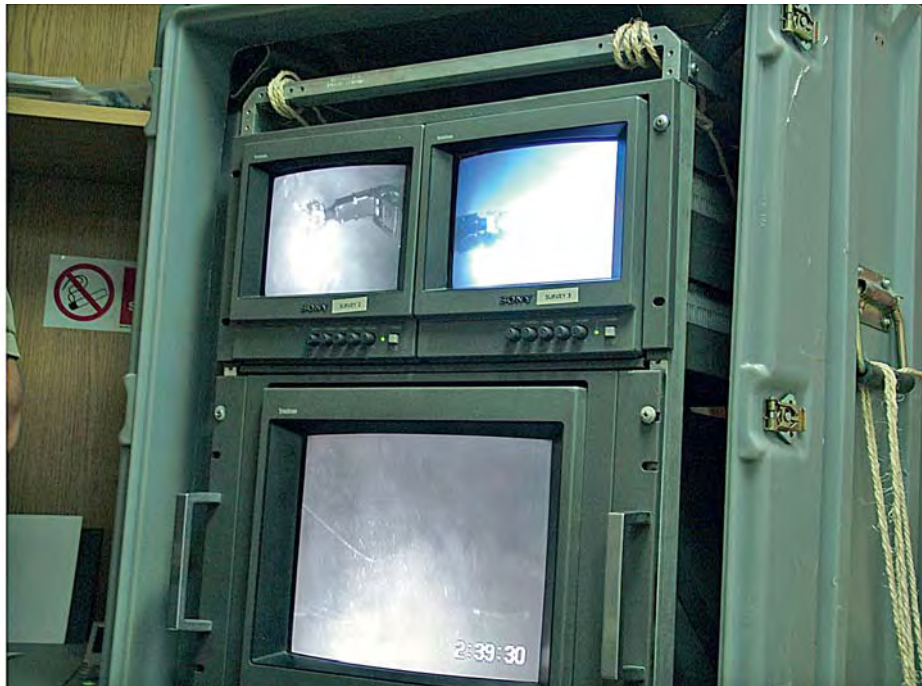
Photo 44: Video system reproducing the images from the video cameras mounted on the ROV.
