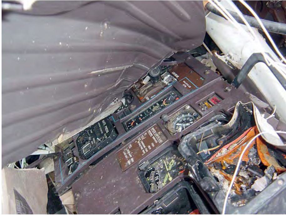
Photo 28: part of the TS-LBB instrument panel after recovery (note the landing gear lever in the “UP” position at the centre of the photo).
