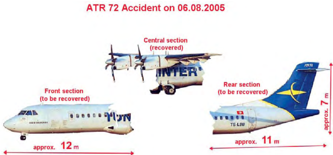
Figure 6: Illustration showing the three sections the aircraft broke into, following impact with the sea surface (ANSV reconstruction). The indication “to be recovered” refers to the date of August 6 th , 2005. These parts were later recovered.
