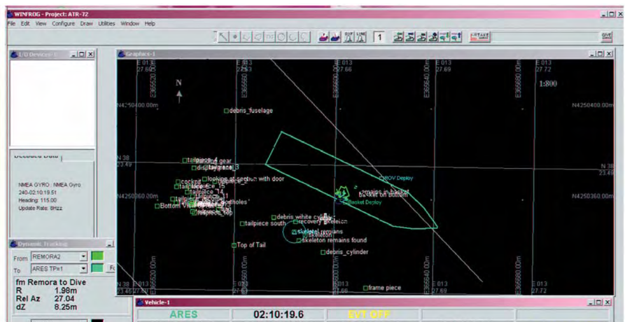
Figure 19: Position of the ship in relation to the parts of the wreckage located.
