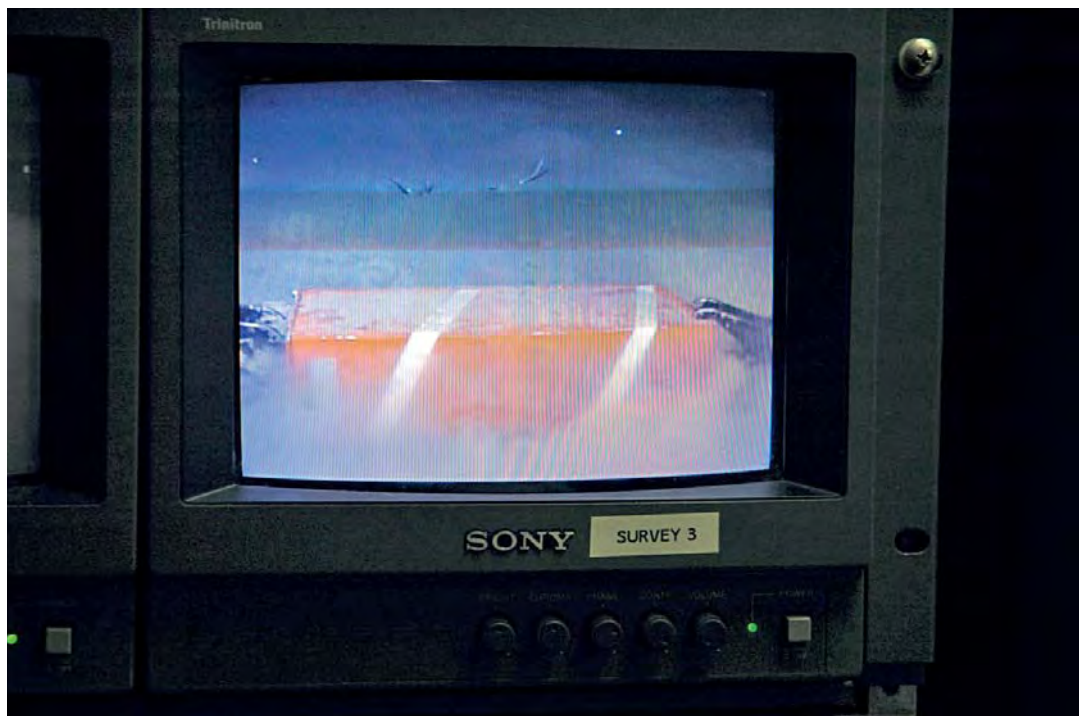
Photo 64: Recovery of the FDR by the ROV.
