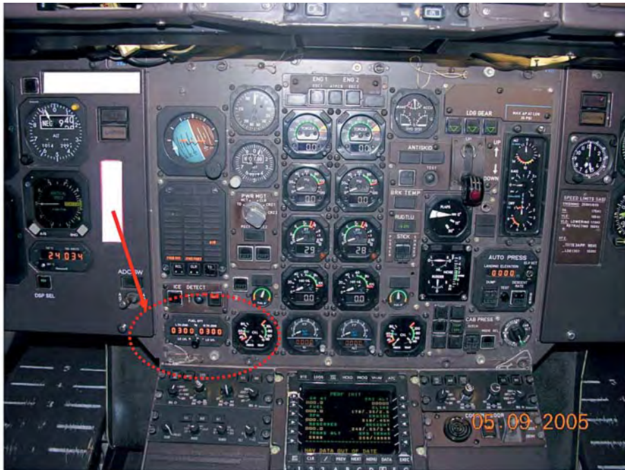
Photo 5: ATR 72 - Center instrument panel – (FQI is indicated by the arrow).
