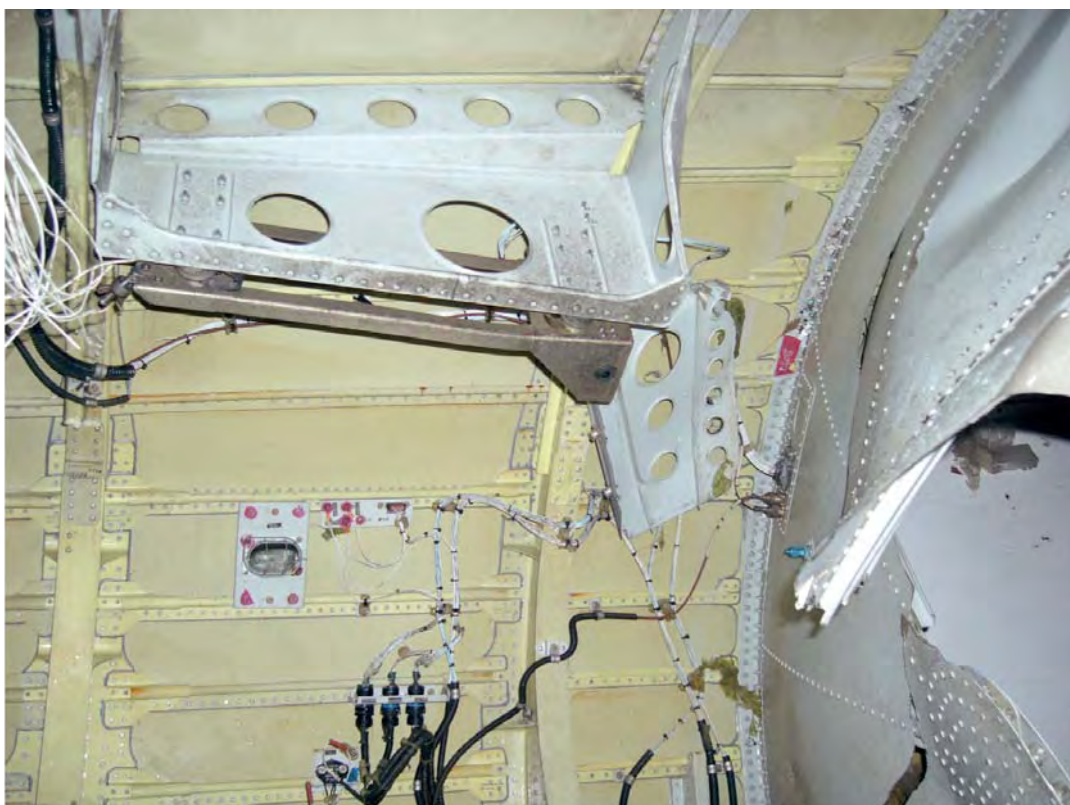
Photo 61: The damaged FDR housing (note the deformation of the pressure bulkhead, demonstrating the strong impact sustained by the rear section of the aircraft).
