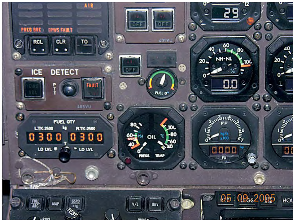
Photo 11: Section of the instrument panel. The Fuel Flow (FF) and Fuel Used (FU) can be seen on the bottom right.
