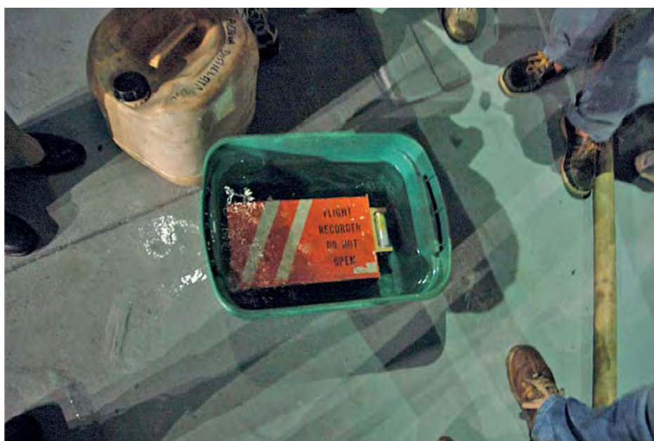
Photo 27: CVR in distilled water, after being recovered from the aircraft.
