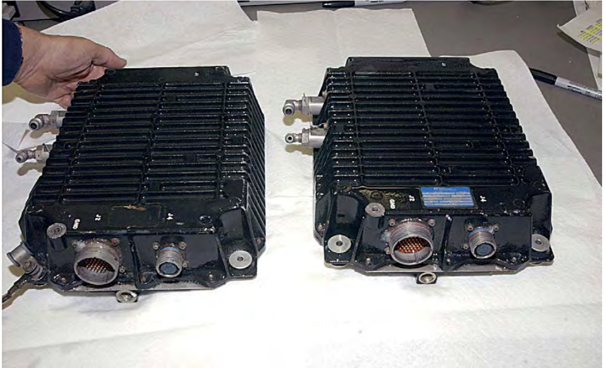
Photo 74: Engine EECs. Note the one on the left, for the right engine, without identification plate.
