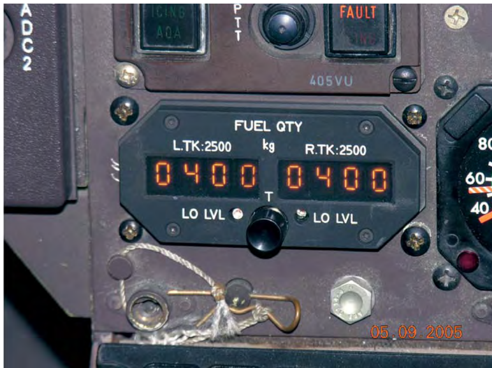
Photo 76: Indication given by ATR 72 FQI fitted on an ATR 72 with 400+400 kg of fuel in each tank.
