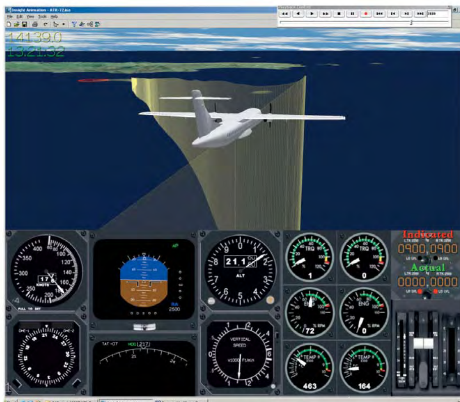
Figure 14: Aircraft during the descent with both engines shut down.
