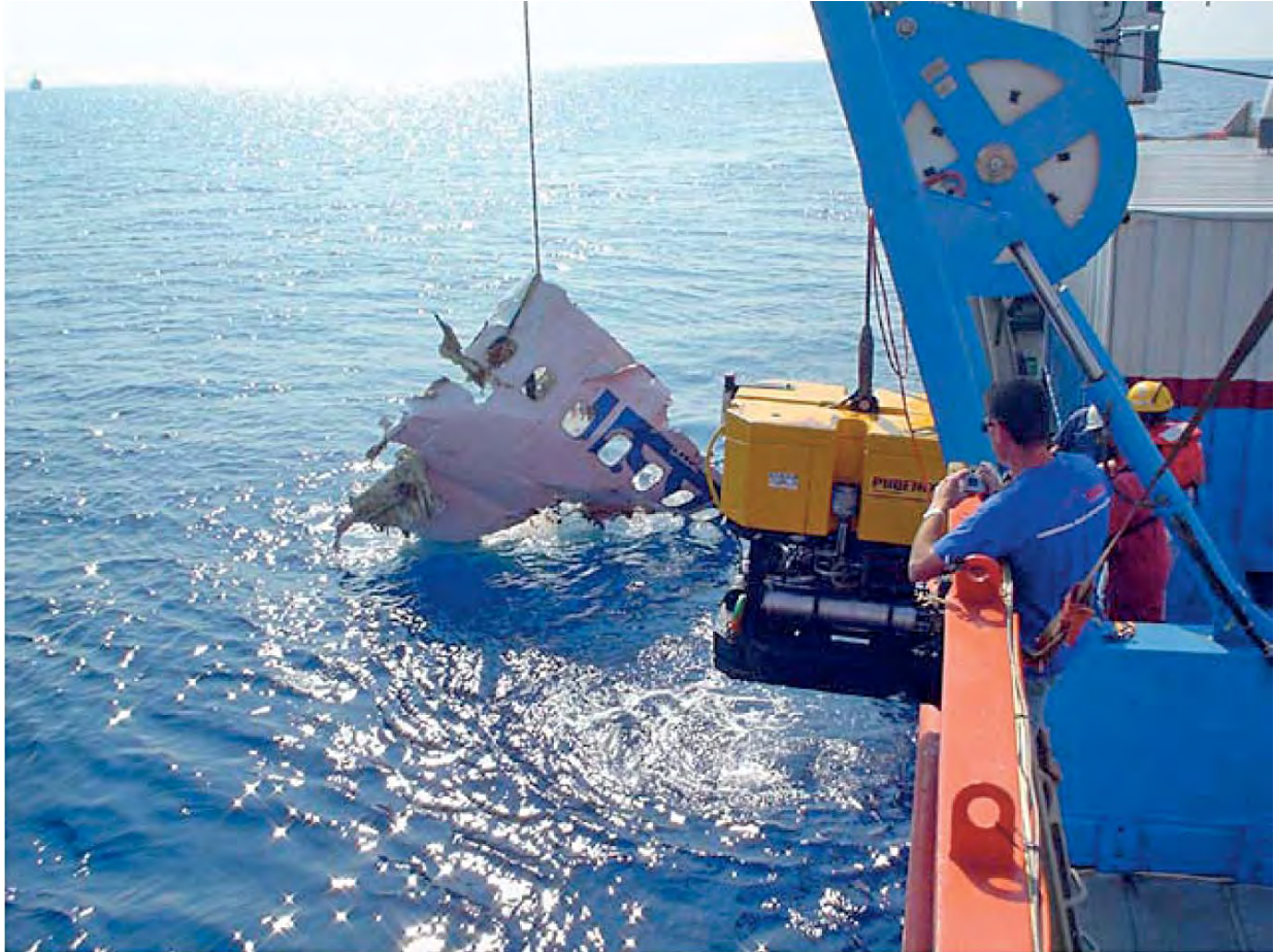
Photo 67: Recovery of aircraft right-hand fuselage panel.
