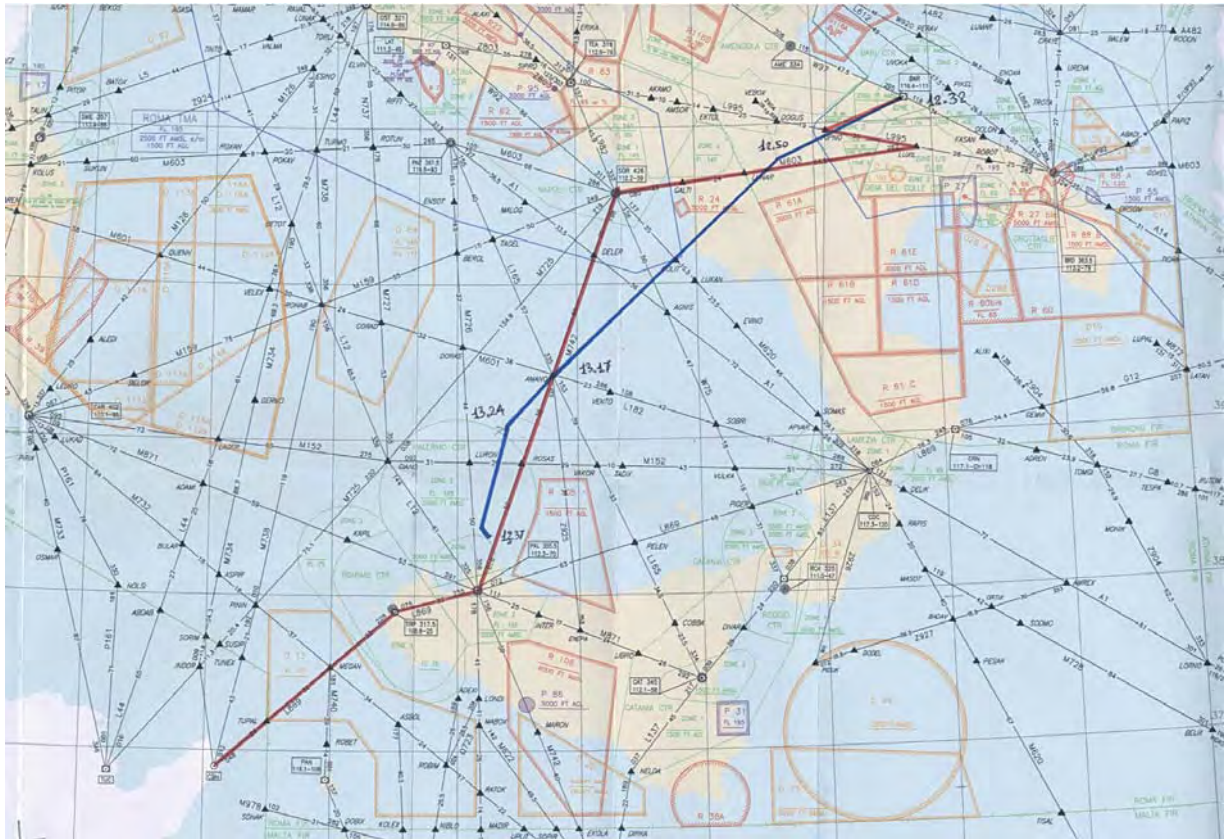
Figure 9: Chart showing the planned route from the flight plan (red line) and the route actually followed by TS-LBB (blue line).
