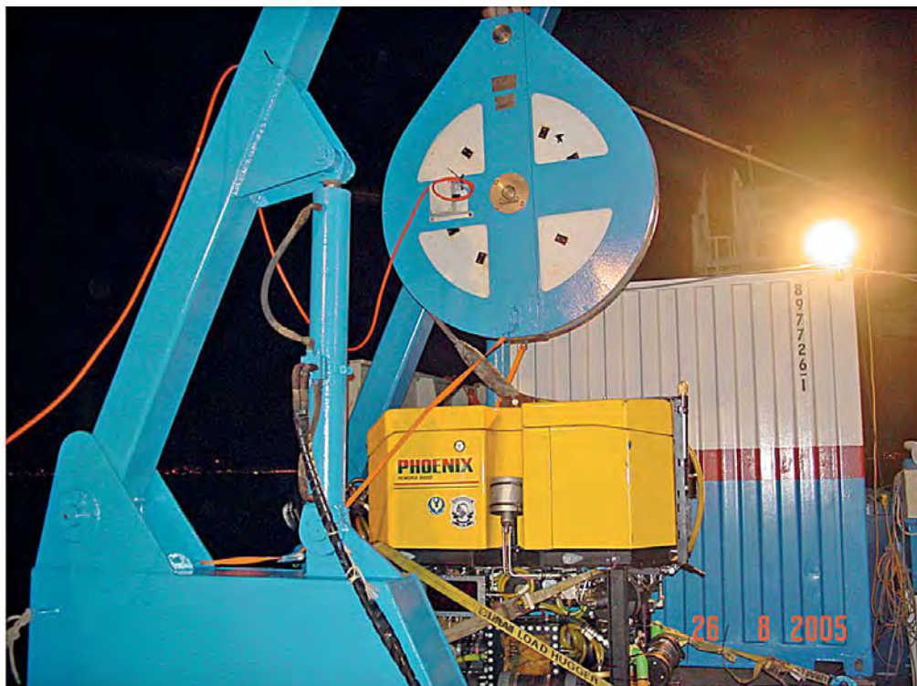
Photo 51: The Remora 6000 on the launching system.
