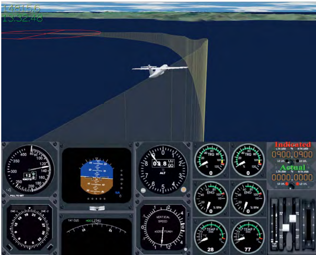
Figure 35: Final phase of the TS-LBB flight path (FDR data).
