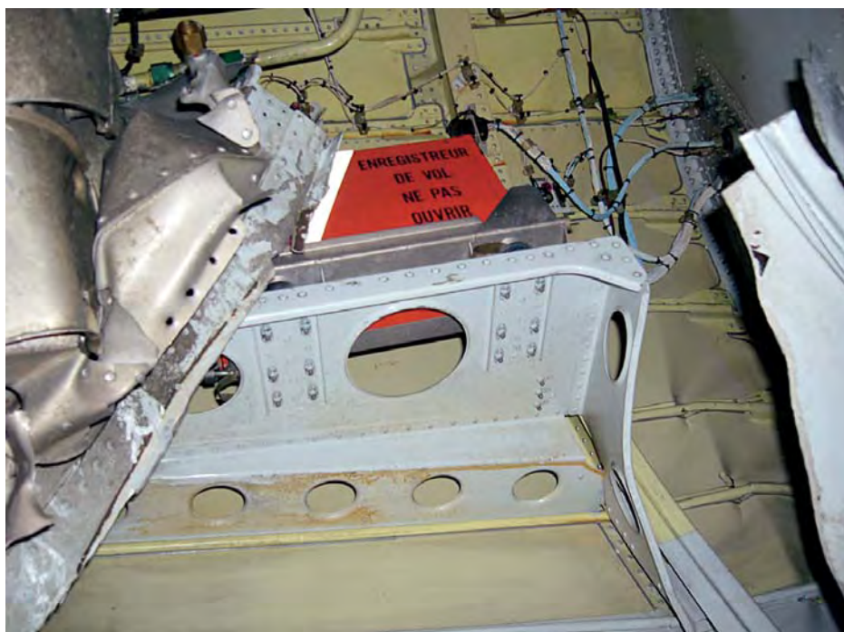
Photo 26: CVR in its housing inside the aircraft.
