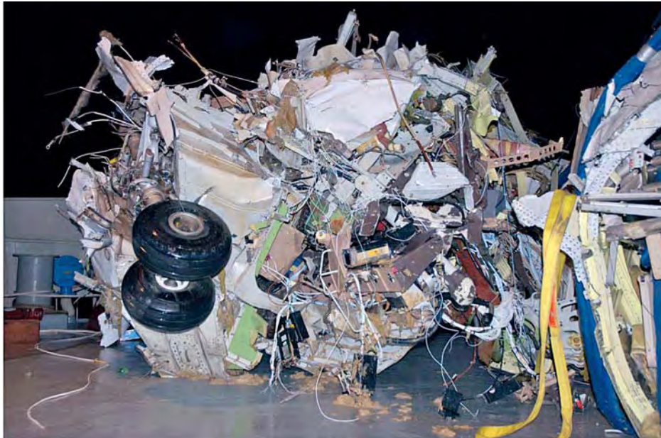
Photo 2: Cockpit soon after recovery from the seabed.
