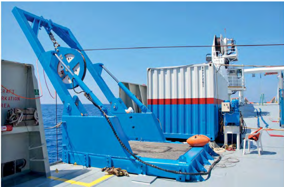
Photo 48: The launching gear used for the Remora 6000.
