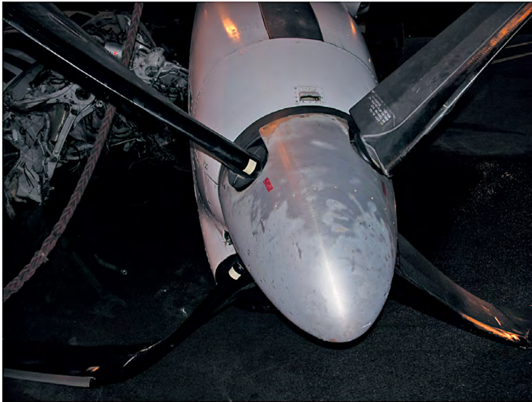
Photo 70: Note the feather position of the right engine propeller.
