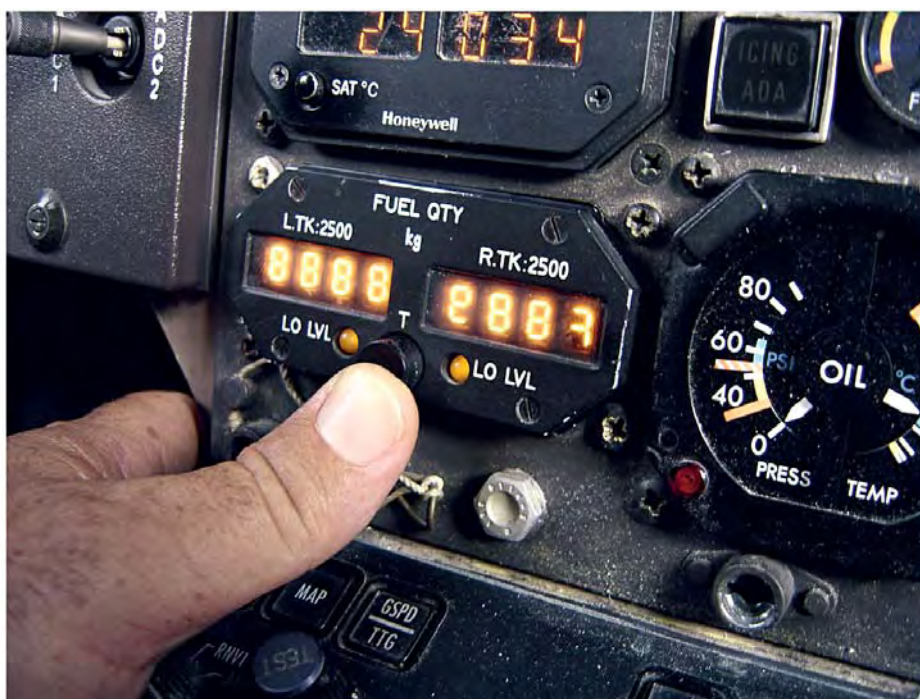
Photo 1: The FQI installed on TS-LBB before replacement.
