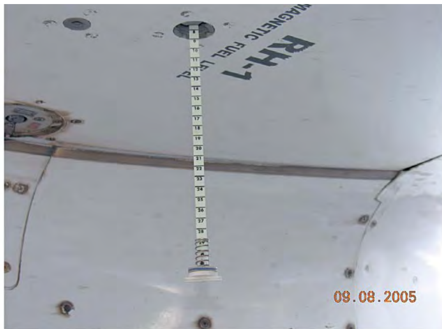
Photo 4: Graduated rod ( dripstick ) for checking the quantity of fuel in the wing fuel tanks.
