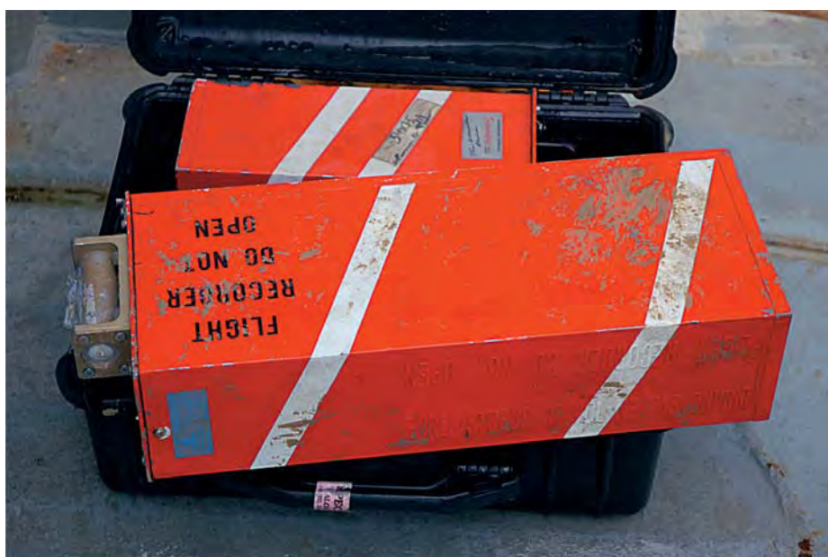
Photo 16: The recovered FDR (foreground) and CVR.
