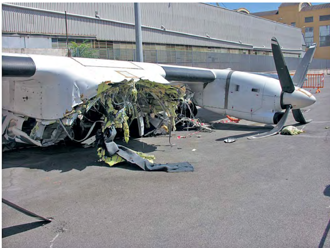
Photo 71: LH and RH wings with part of the central fuselage and engines after recovery.
