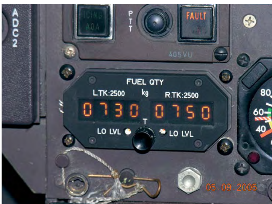
Photo 79: Indication given by the FQI ATR 72 on an ATR 72 with approximately 3800 kg selected (total actually present equals to approximately 1500 kg).
