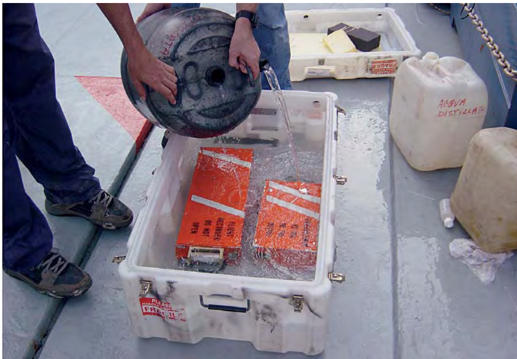
Photo 66: FDR (on the left) and CVR (on the right) immersed in distilled water for preservation and transport purposes.
