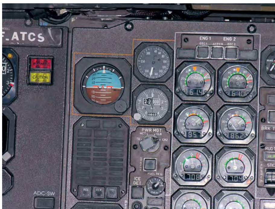
Photo 85: Detail of stand-by instruments.
