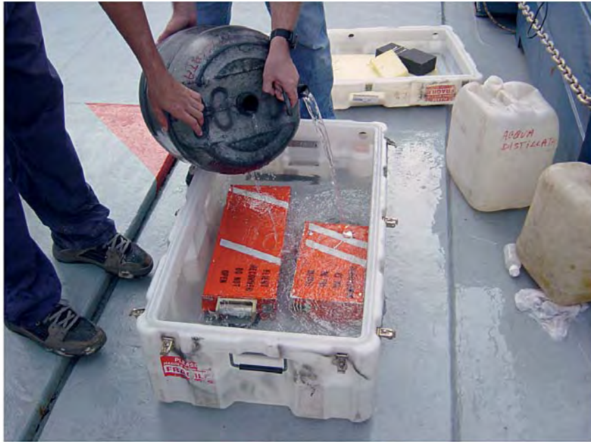
Photo 17: Preservation of the FDR and CVR in distilled water.
