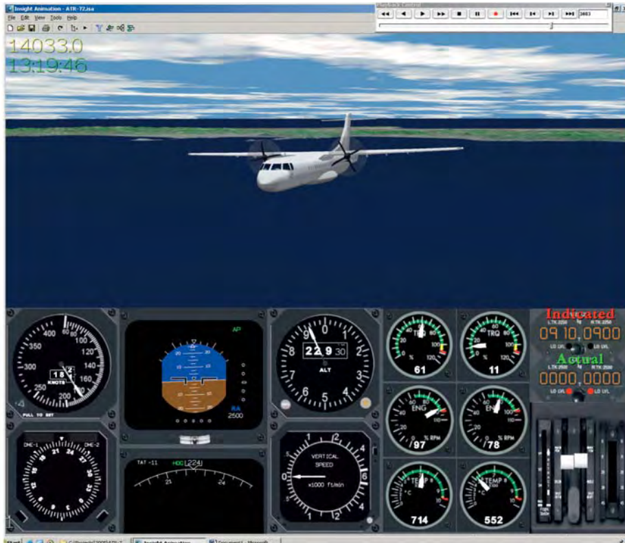
Figure 13: Right engine shut down.
