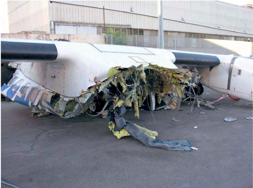
Photo 72: LH and RH wings and engines after recovery, the central fuselage section, front view.
