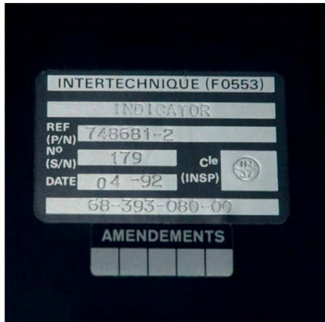
Photo 80: FQI S/N 179 nameplate (Data Plate).
