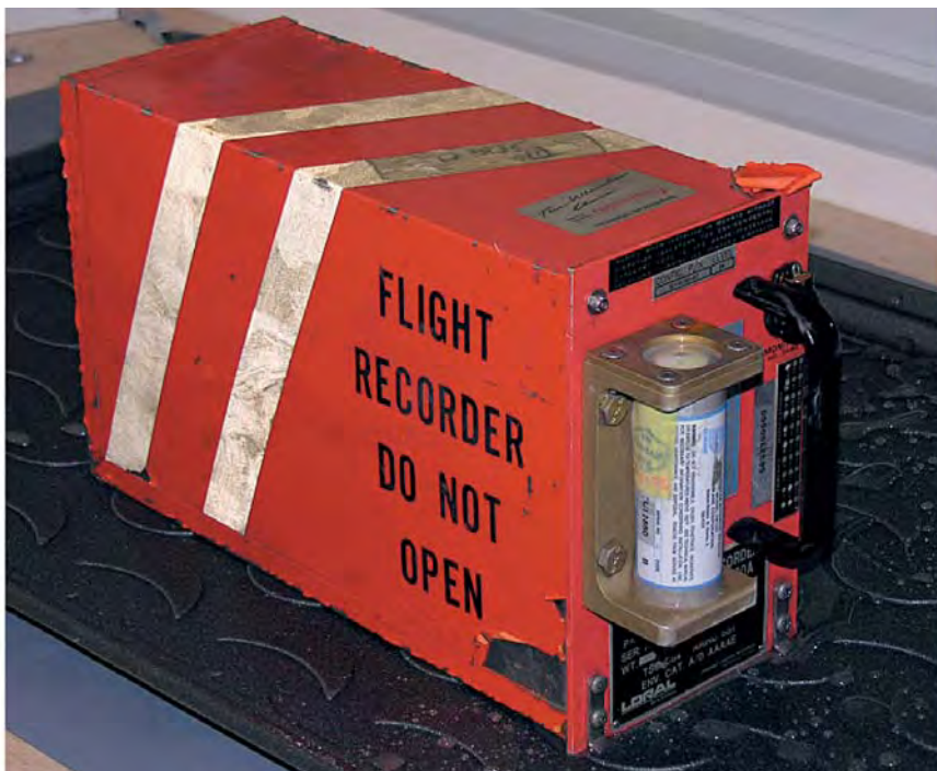
Photo 18: CVR, external condition. ULB in foreground.
