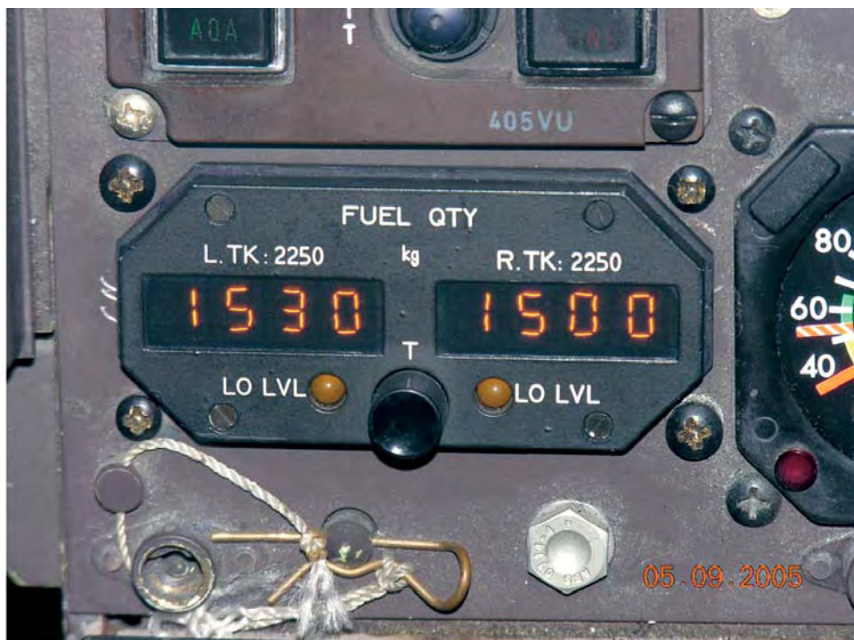
Photo 77: Indication given by an ATR 42 FQI fitted on an ATR 72 with 400+400 kg of fuel in each tank.
