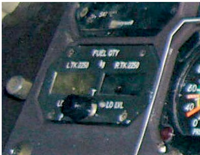
Photo 87: FQI installed onboard TS-LBB, taken immediately after wreckage recovery.
