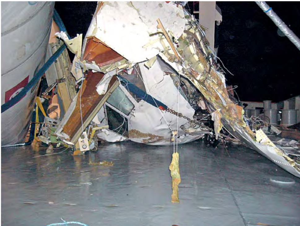
Photo 37: Part of the cockpit immediately after recovery.
