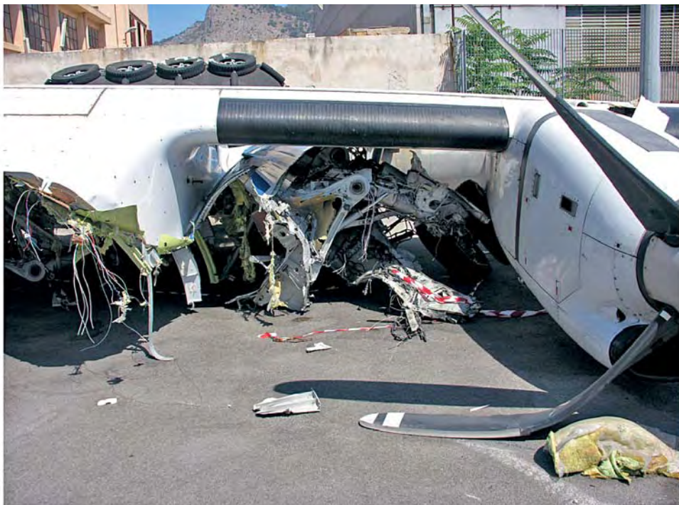
Photo 23: Part of the central fuselage with LH and RH wings at the Port of Palermo, the central section.
