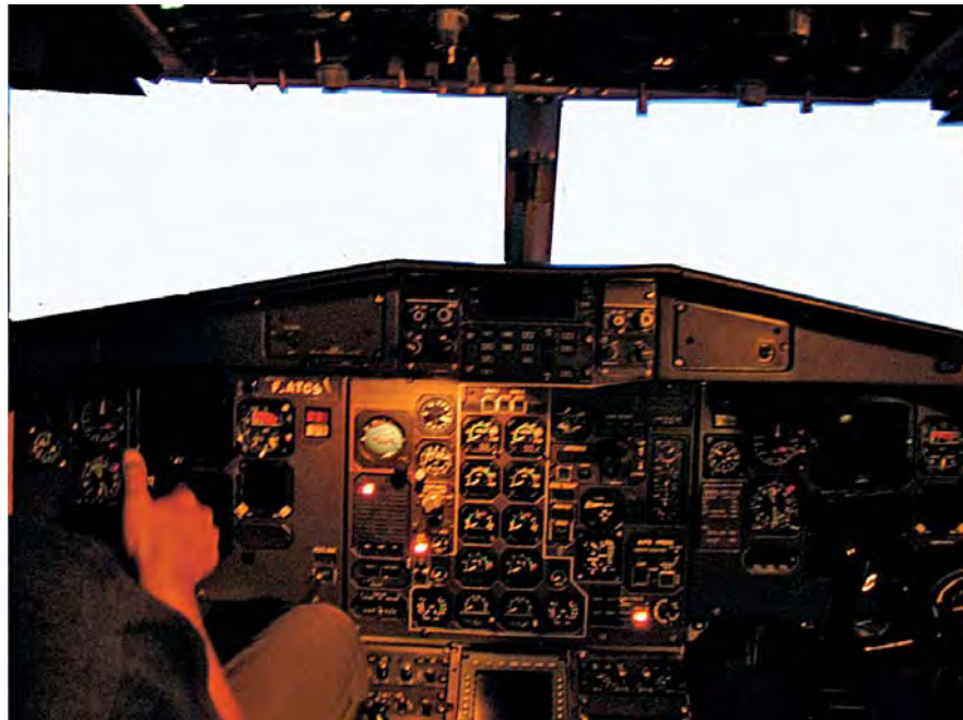
Photo 86: Tests on the simulator, note the stand-by instrument panel (illuminated).
