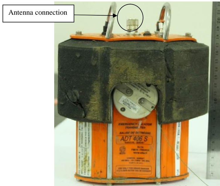
Figure 21: Emergency Locator Transmitter with antenna detached
