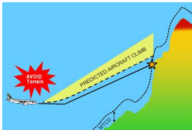
Figure 2: TAWS looking forward function using flight path angle and aircraft climb model: Avoid Terrain Warning
