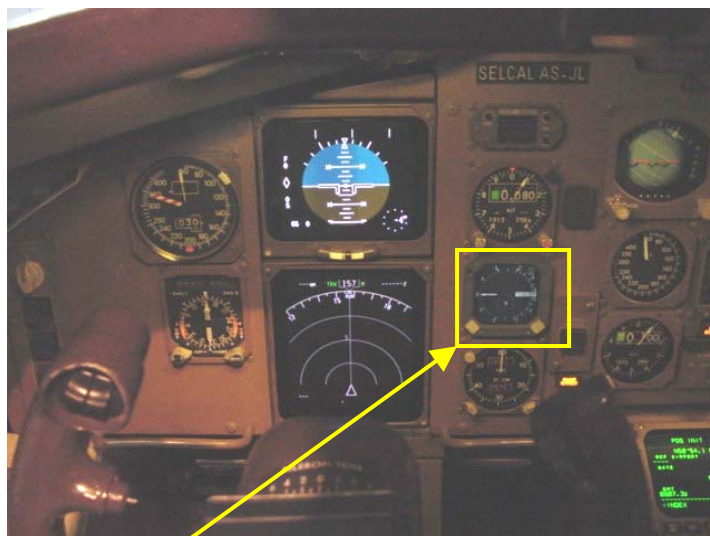
Position of the VSI/TRA in the B757-200 cockpit
