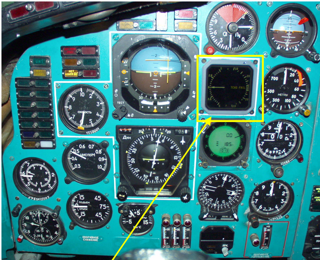
Position of the VSI/TRA) in the TU154M cockpit
