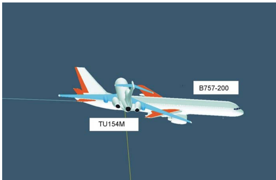
Reconstruction of the collision according to FDR data and collision evidence
