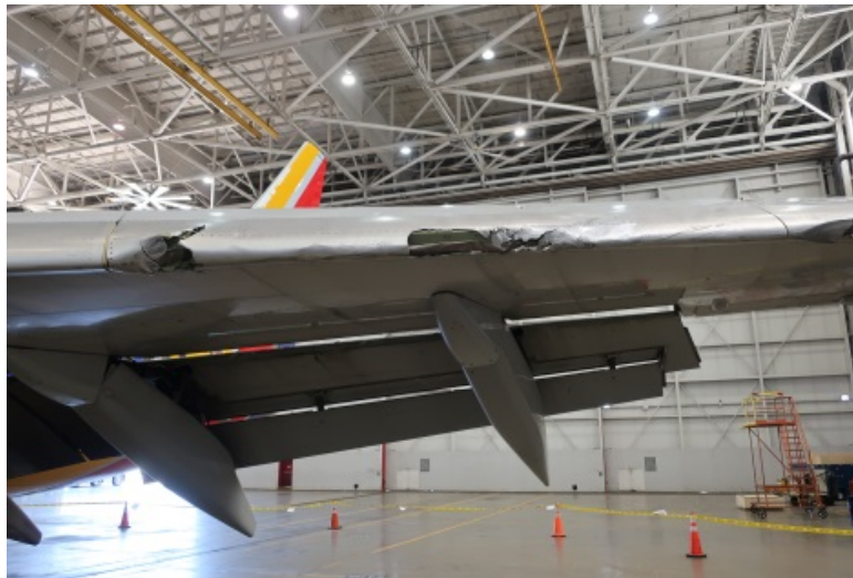
Figure 3. Damage to leading edge of left wing
