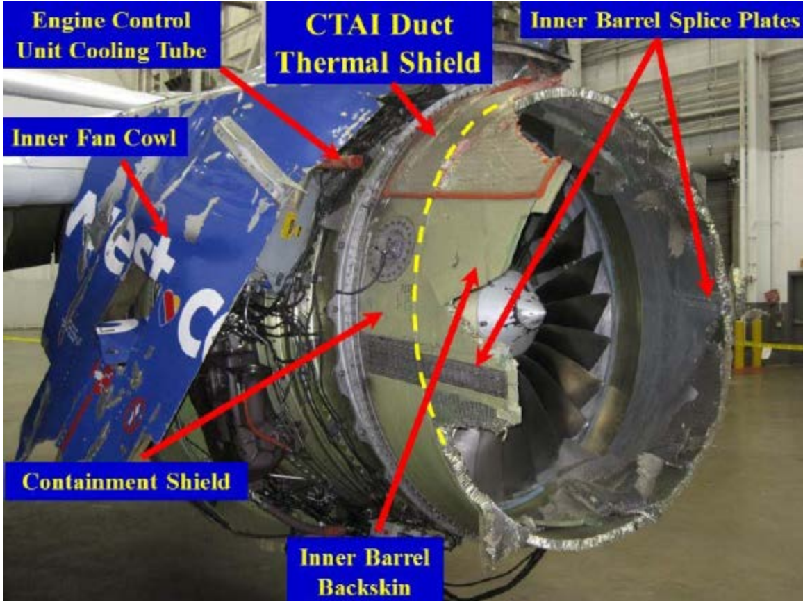
Figure 1. Damage to cowl - inboard
