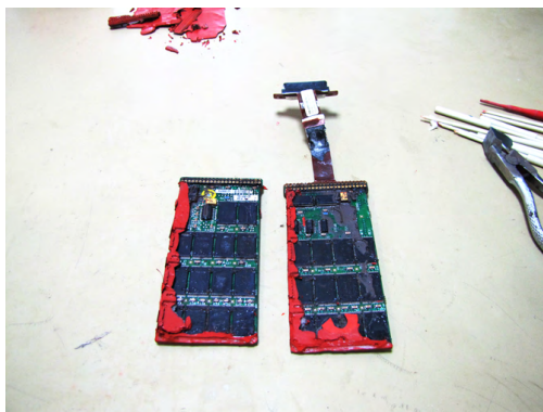
CVR memory boards after cleaning
