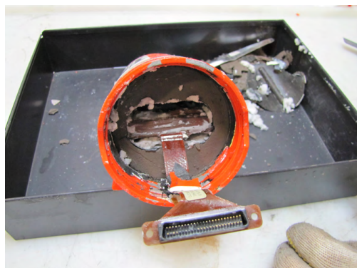
CVR memory board after removal of thermal protections
