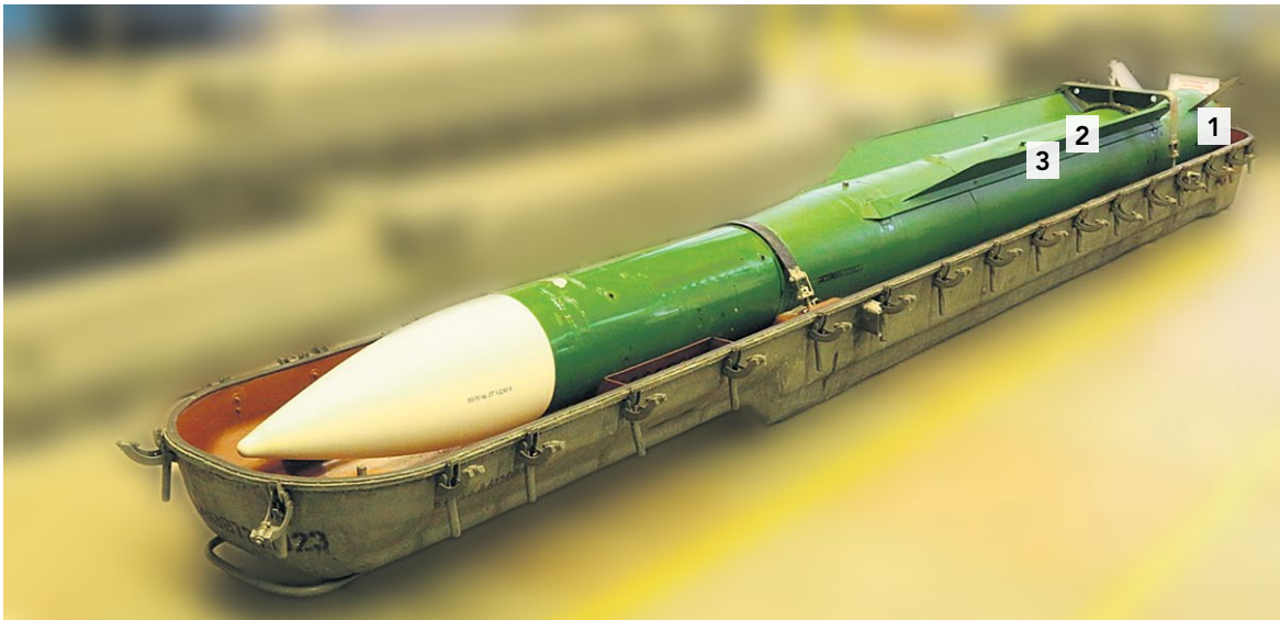
Figure 35: Image of 9M38M1 surface-to-air missile showing the approximate location of three of the parts recovered. (Source: NBAAI)
