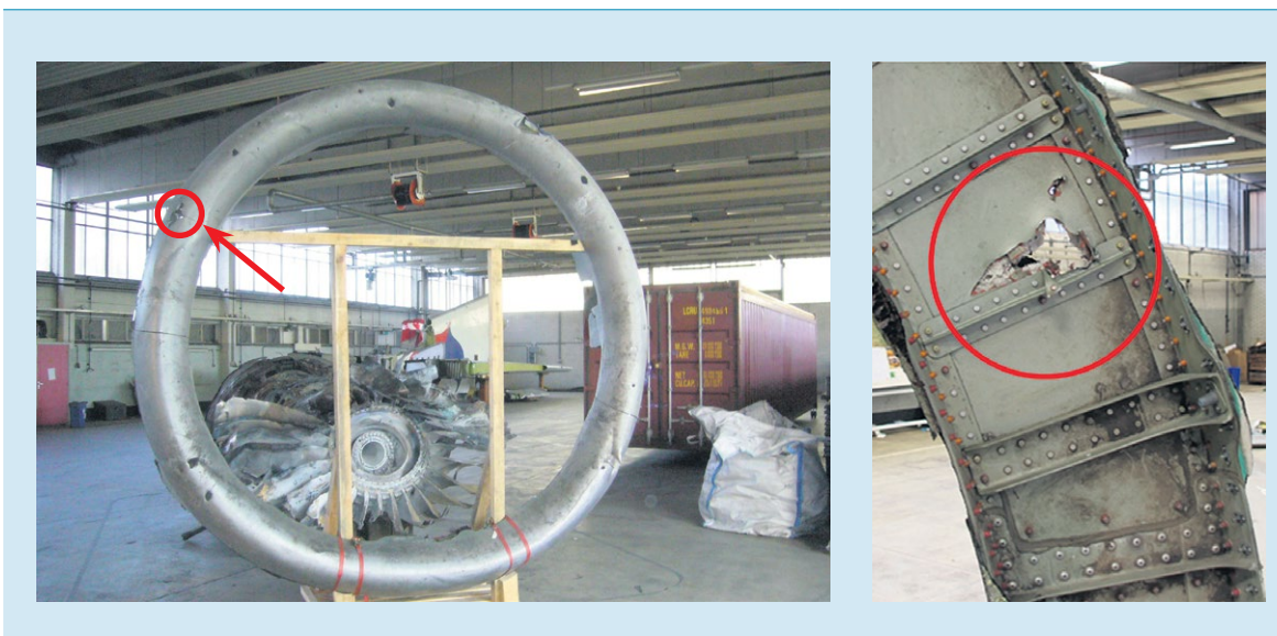
Figure 17: Damaged left engine intake ring, with impact marks seen from the front side (left photo) and from the rear side (right photo). (Source: Dutch Safety Board)
