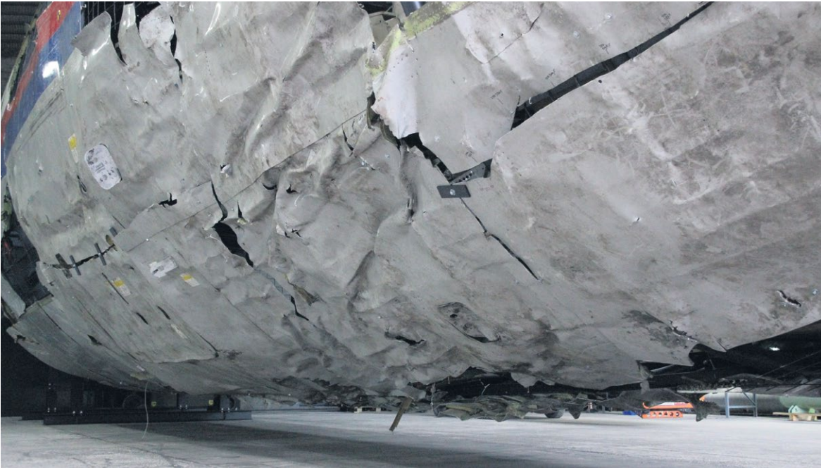
Figure 23: Fuselage skin pushed in between stringers and frame. (Source: Dutch Safety Board)
