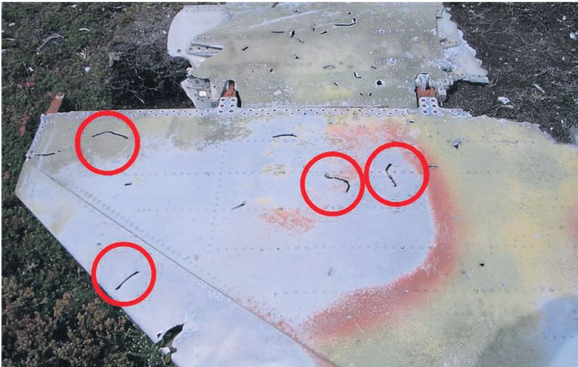
Figure 52: Example of damage caused by metal rod warheads. (Source: PPRuNe, via NLR)
