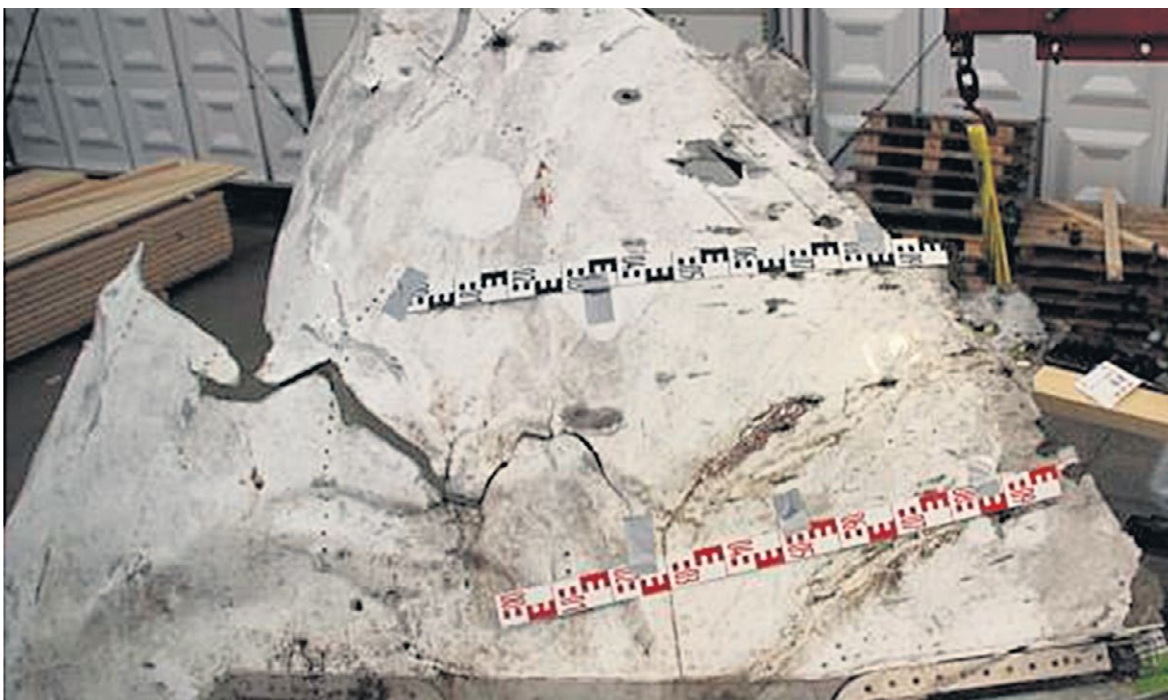
Figure 49: Grazing on cockpit roof. (Source: NLR)
