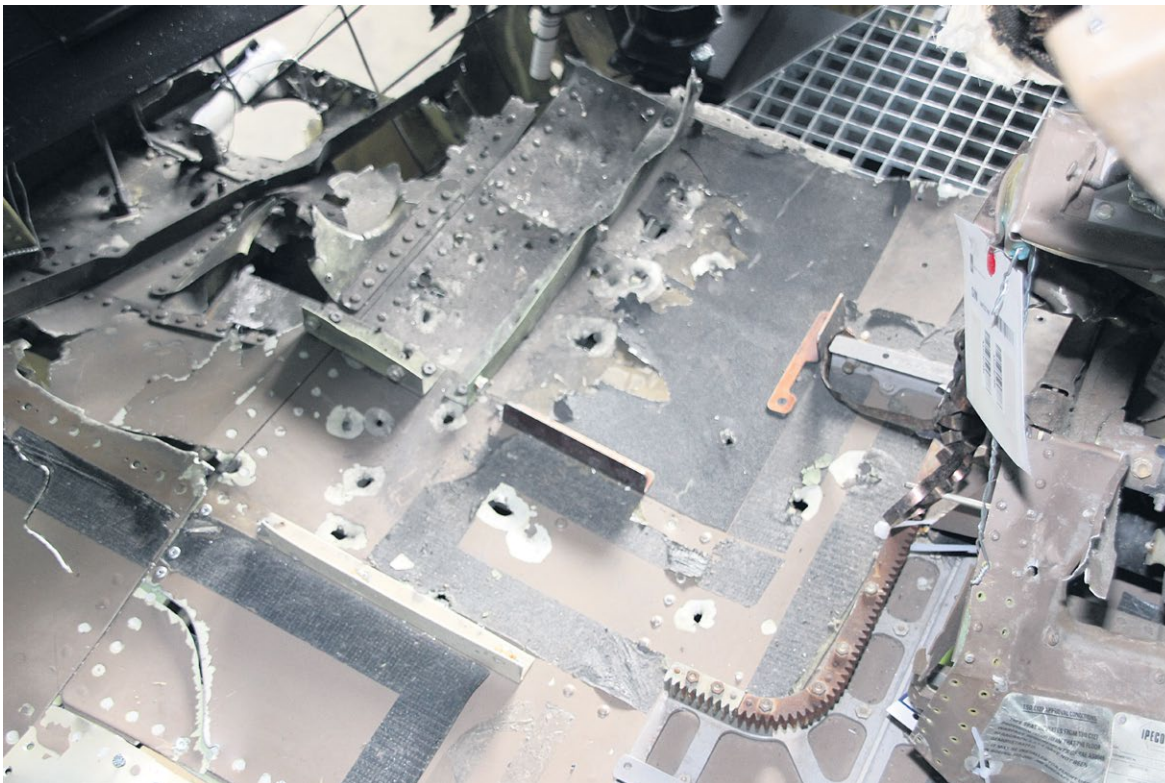
Figure 22: Cockpit floor with floor parts showing perforation holes. (Source: Dutch Safety Board)
