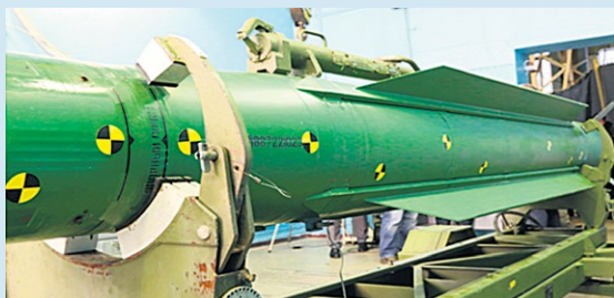
2. Stabilizing fins. (Source: NBAAI)
