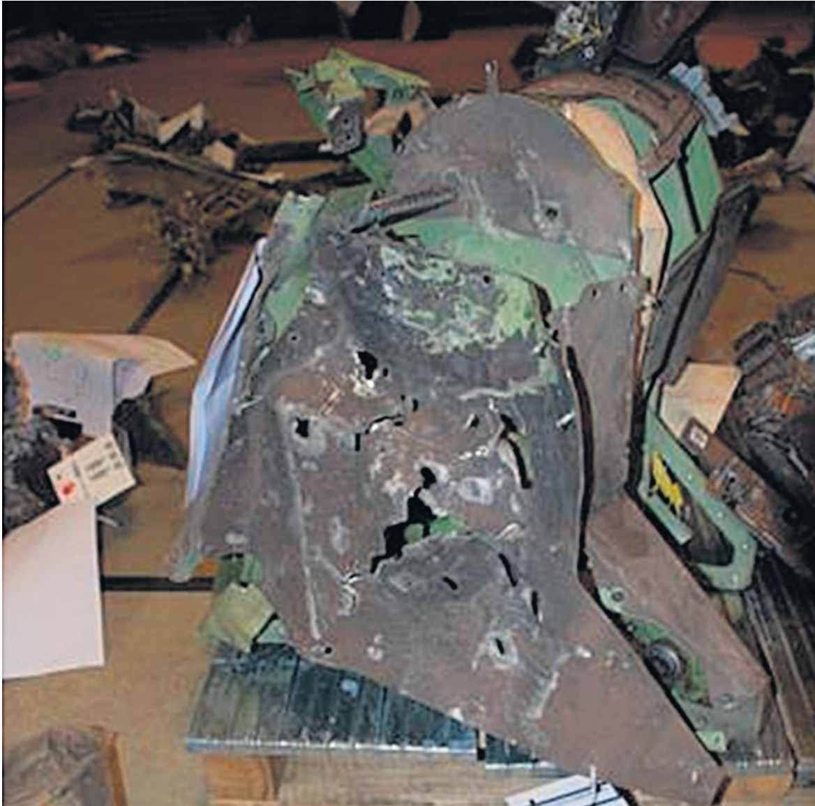
Figure 25: Throttle quadrant (viewed from the left hand side) showing perforation damage. (Source: NLR)
