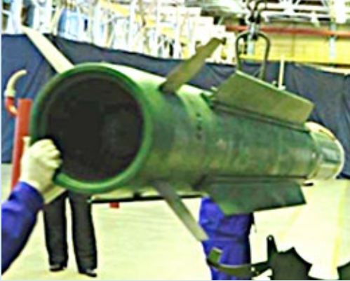
1. Rear nozzle of the missile's engine. (Source: NBAAI)
