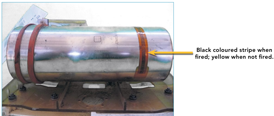
Figure 75: One of the recovered passenger oxygen generators. (Source: Dutch Safety Board)
