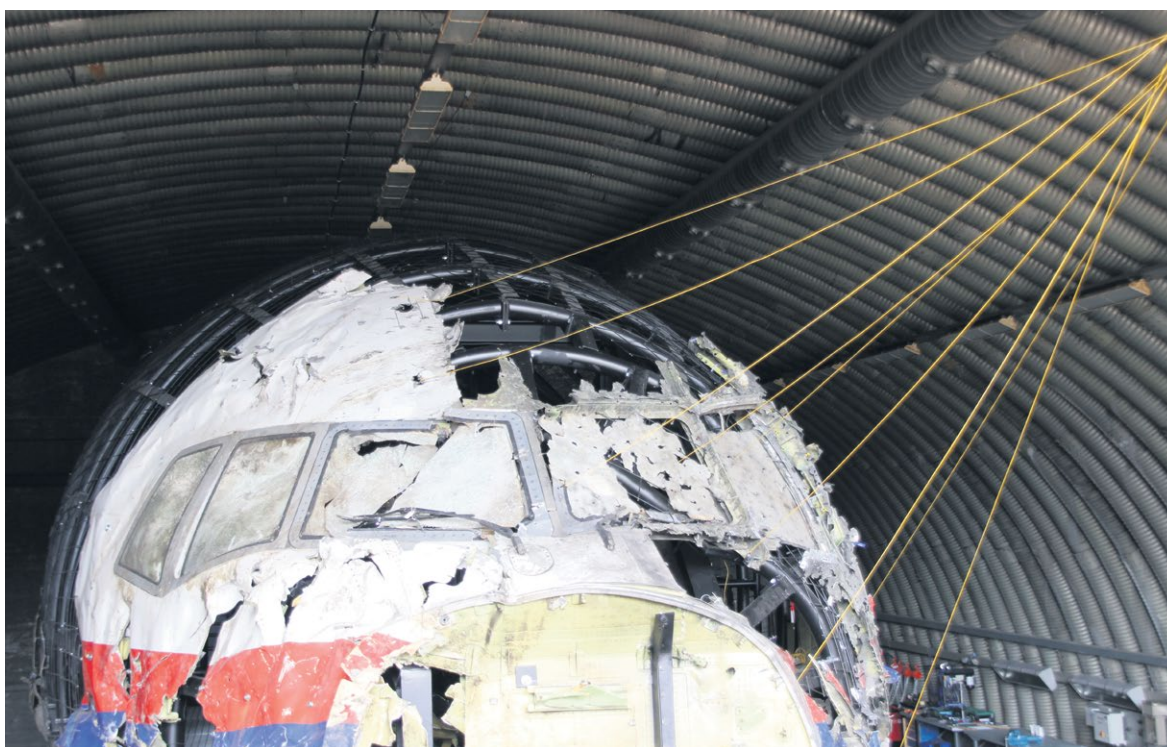
Figure 50: Impression of stringing of the cockpit. (Source: Dutch Safety Board)
