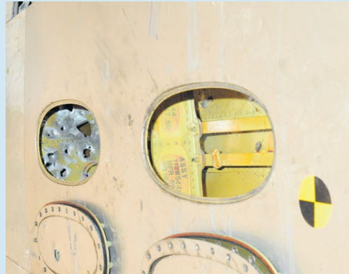
Location of the fragment inside the left wing tip, seen from below. (Source: Dutch Safety Board)
