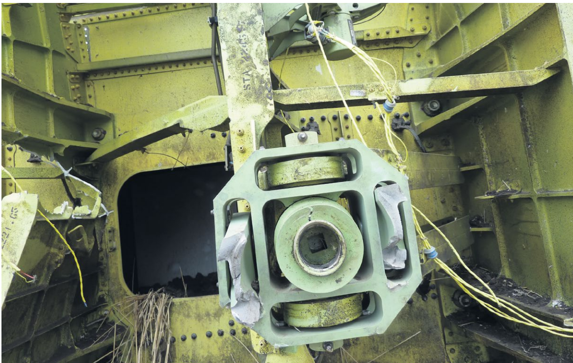
Figure 72: Overload failure of the vertical stabilizer. (Source: Dutch Safety Board)
