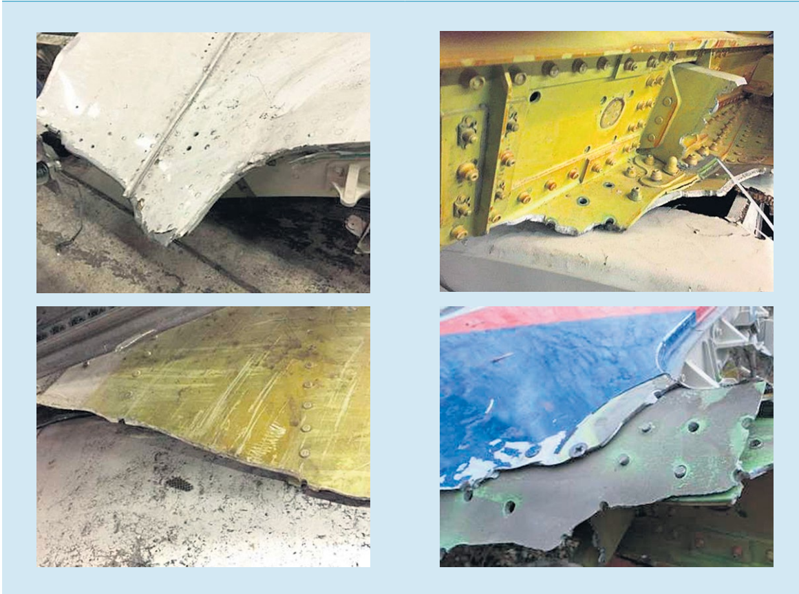
Figure 69: Examples of tensile overstress fracture at passenger doors 3L and 3R. (Source: Dutch Safety Board)
