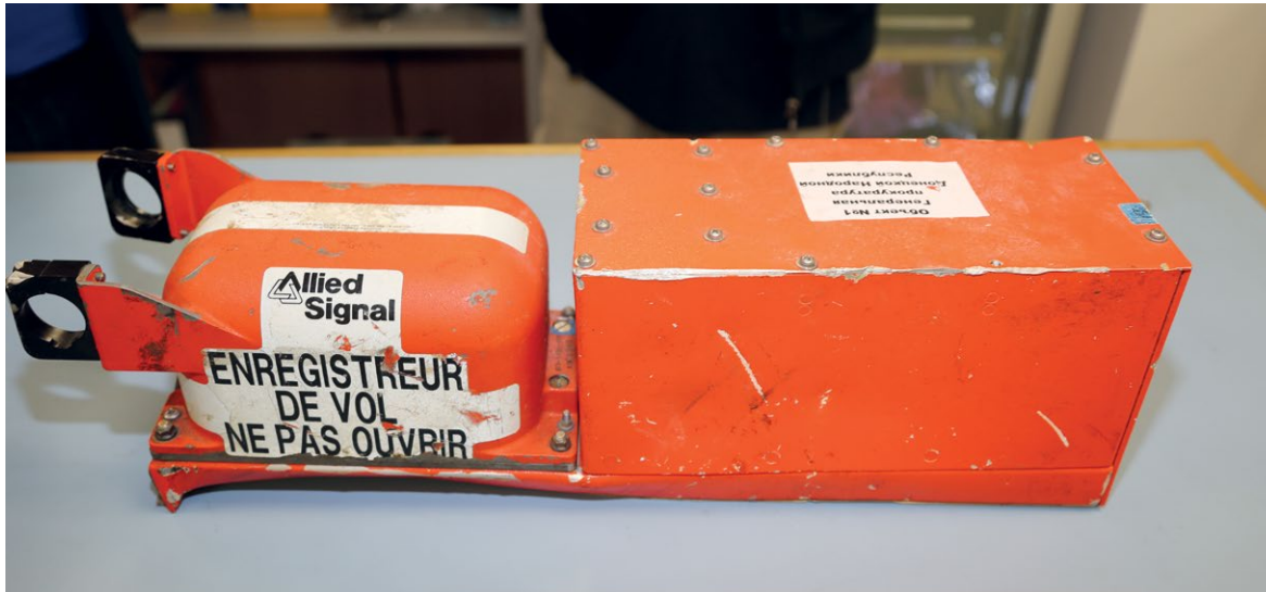
Figure 10: Flight data recorder without Underwater Locator Beacon. (Source: Dutch Safety Board)
