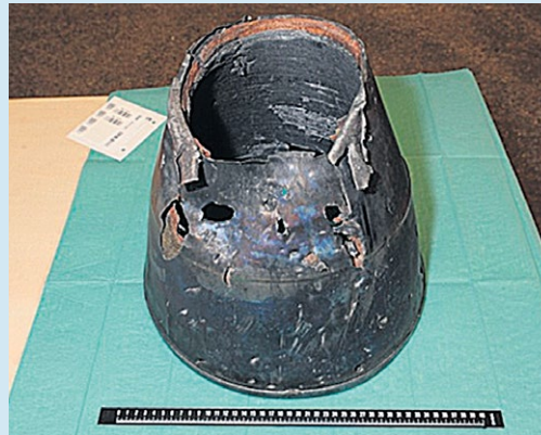
Missile engine nozzle as found in Ukraine. (Source: Dutch Safety Board/Dutch National Police)
