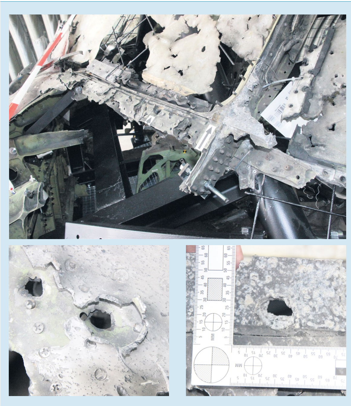
Figure 47: Part of the left hand cockpit window frame with enlarged detail. The perforation damage had a regular pattern of larger and smaller holes. (Source: Dutch Safety Board)
