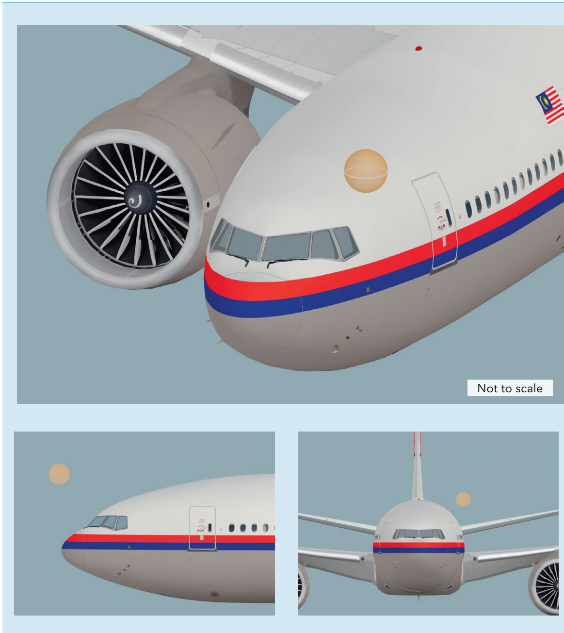
Figure 61: Simplified representation of the volume of space of the warhead detonation location according to three independent simulations. (Source: Dutch Safety Board)
