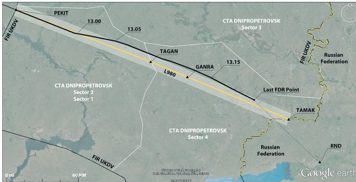
Figure 85: Image of the Dnipropetrovsk FIR (UKDV), CTA 1 and 4, and the flown (black line) and intended (dotted black line) route of flight MH17. The yellow line represents the centre of airway L980. (Source: UksATSE and Google, Landstat)
