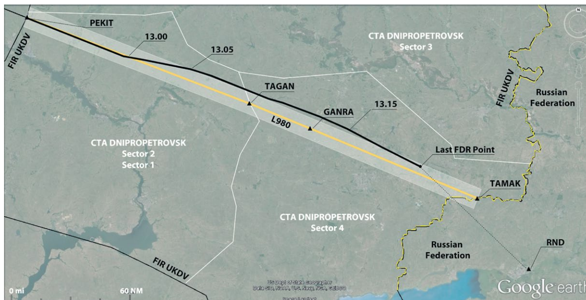
Figure 3: Route of flight MH17 across the eastern part of Ukraine. The light grey shading shows the area that is 5 NM left and right of the centreline of airway L980. The black line shows flight MH17 deviating from airway L980 between air navigation waypoints PEKIT and TAGAN. (Source: Google, Landstat)
