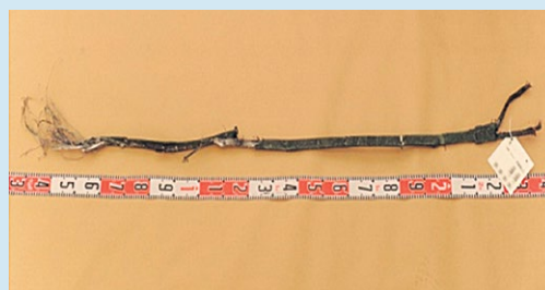
Data cable during identification at Gilze-Rijen Air Force Base. (Source: Dutch Safety Board/Dutch National Police)
