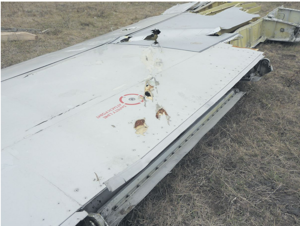
Figure 29: Left wing tip with impact damage near and outboard of the safety line attachment point. (Source: Dutch Safety Board)
