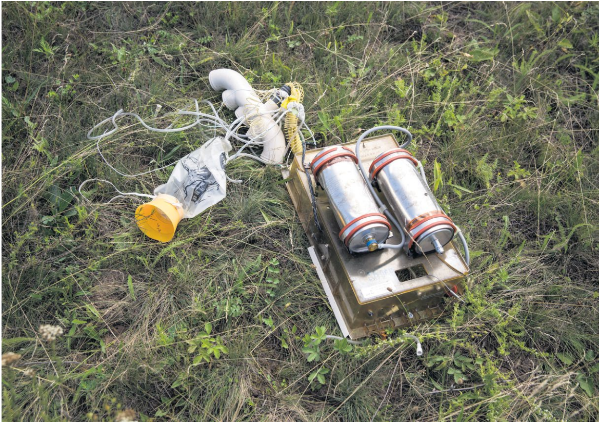
Figure 41: Chemical oxygen generators and part of the passenger service unit. (Source: Dutch Safety Board)
