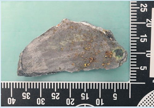
Metal fragment recovered from inside the left wing tip. (Source: Dutch Safety Board/Dutch National Police)
