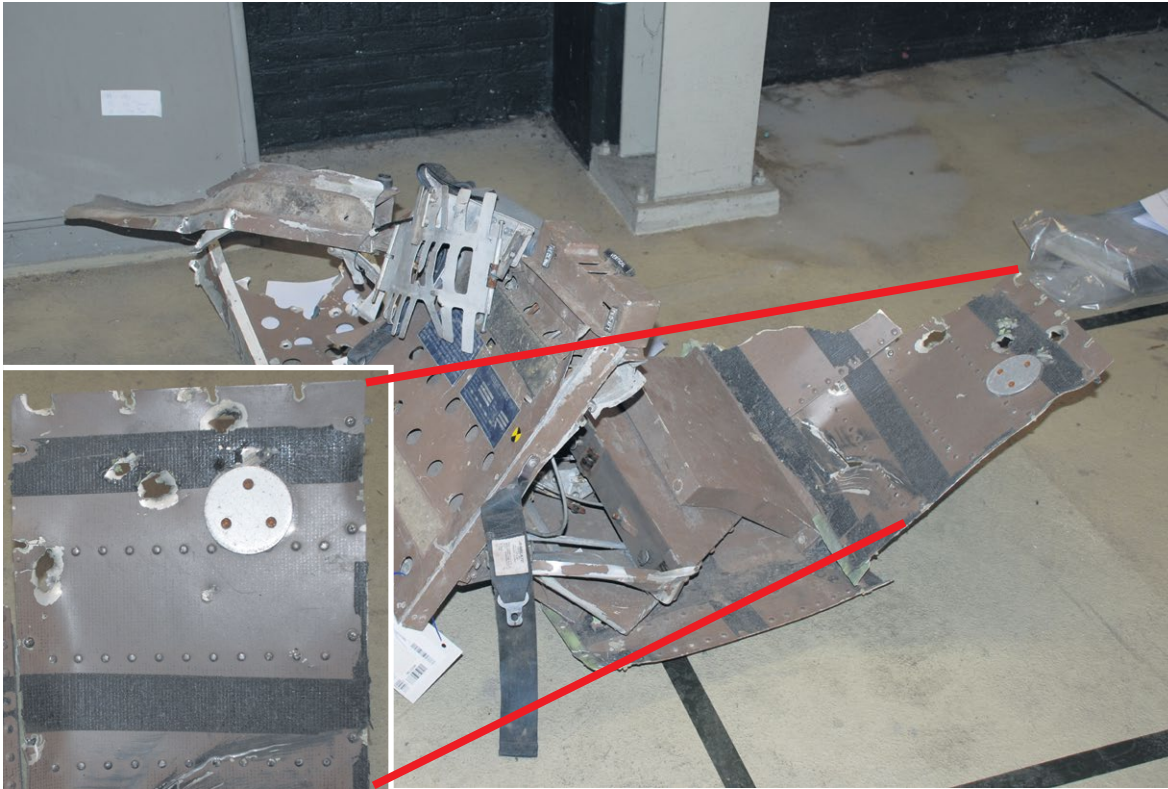
Figure 27: Perforation holes in seat back panel of left observer seat. Note: The seat back panel is shown flat on the floor in this image. (Source: NLR)
