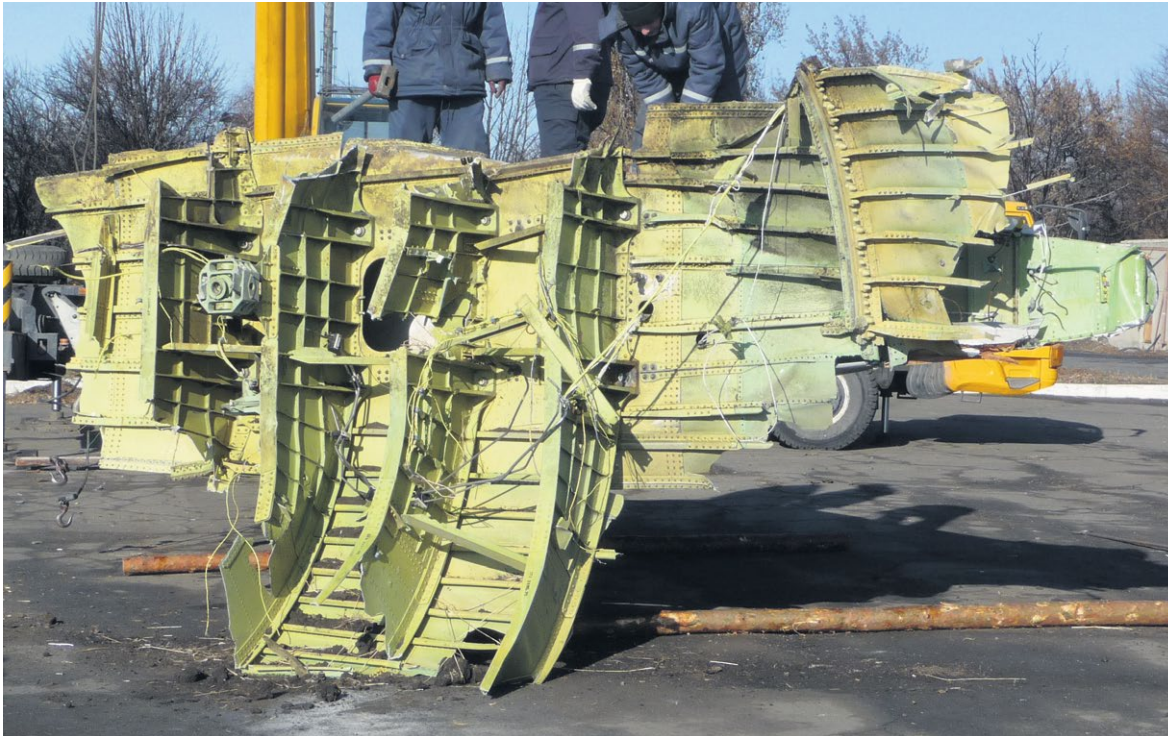
Figure 73: Fracture separating the vertical stabilizer from the fuselage. Attached skin and broken vertical stabilizer-to-fuselage frames bended out of their plane and fractured. (Source: Dutch Safety Board)
