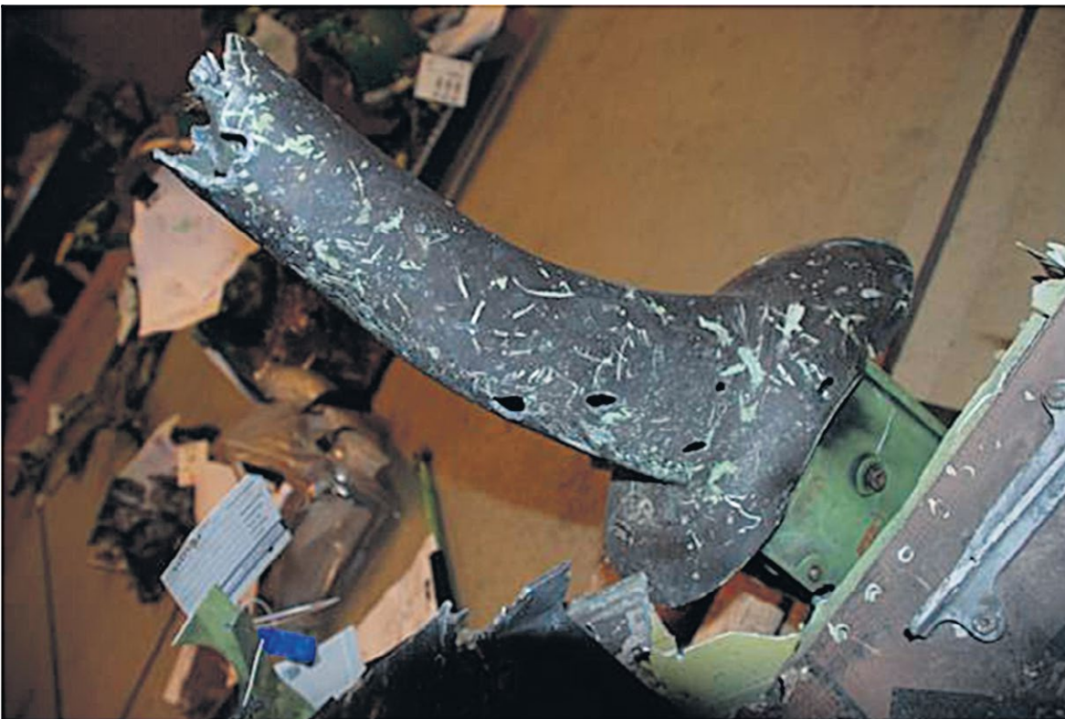
Figure 24: Lower part of Captain's control column showing perforation damage. (Source: NLR)
