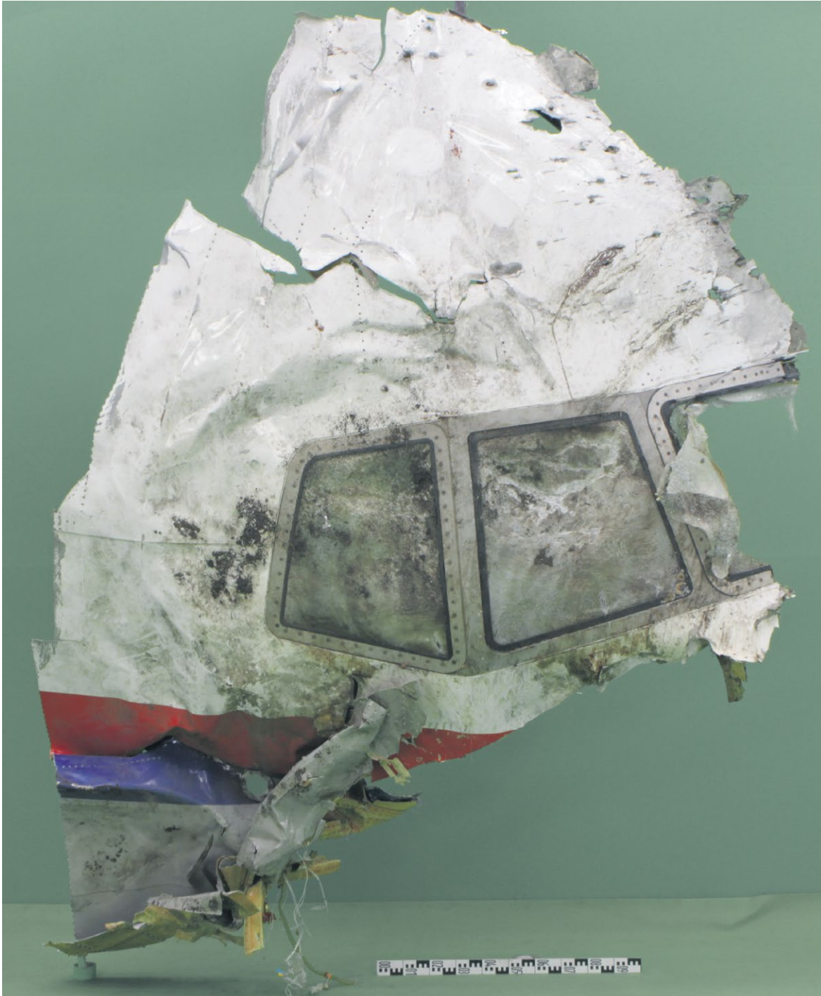
Figure 19: Part of the right hand side of the cockpit. (Source: Dutch Safety Board)
