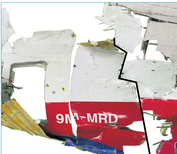
Figure 70: Left hand side separation fracture between rear fuselage and the tail. Separation is at the irregular fracture indicated by the black line. The vertical cut through the left letter M was made for transportation purposes. (Source: Dutch Safety Board)
