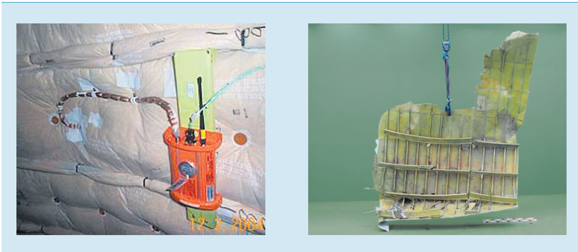
Figure 11: Fixed ELT location installed in a Boeing 777 (left), panel recovered from 9M-MRD with no insulation material or ELT attached (right). (Source: Dutch Safety Board)
