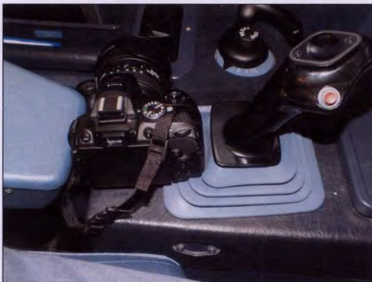
Figure 8: Re-construction of Captain's camera behind side-stick.
