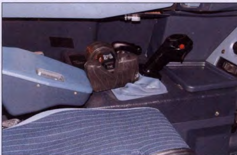
Figure 9: Side-stick locked in fully forward position (substitute camera).
